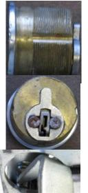
Mortise lock cylinders are threaded like a large machine screw with fine threads and are held in place by a small set screw. These fine threads make these cylinders easy to pull with a lock-pulling tool. Once the cylinder is removed you will need to replicate its action with a key tool. The cam on the back of the cylinder that rotates when turned with the key indicates the use of the bent end of the key tool.
